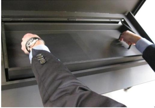
Now the ash drawer can be withdrawn using both handles. When re-installing the ash drawer, make sure that the rear of the ash drawer is positioned underneath the support face. Only the sides and front of the ash drawer are supported.
