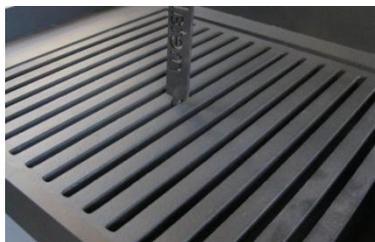
Turn the key 90° so that it is secured between the grooves of the grate. Now the grate can be lifted up with the door handle.
