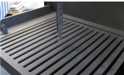
Position the door handle in the groove of the grate.
